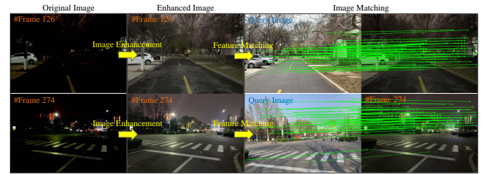
Fig. 1. The contrast results reveal some details in dark areas before and after image enhancement. The proposed end-to-end dark-enhanced Net performs feature matching and image matching successfully.
